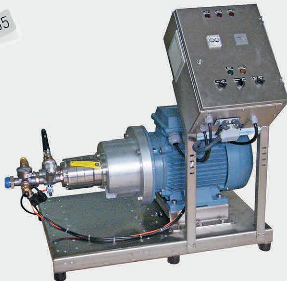
DFP32-45 45 LPM 100 BAR DANFOSS 400 V 215 Kg ALL SS FRAME Control Box, On-Off timer, Pressure Switch, Automatic Drain
