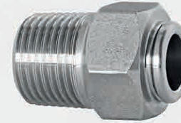
Stainless Steel 3/8" male connector for 3/8" tube NPT 303 quality
