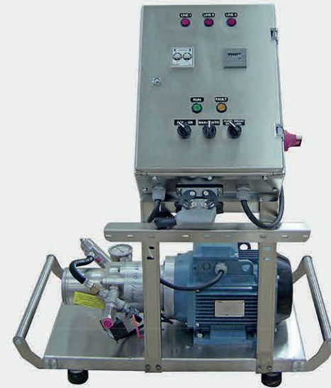
DFP-10-13 13LPM 100 BAR DANFOSS 400V 61 Kg ALL SS FRAME Control Box, On-Off timer, Pressure Switch, Automatic Drain
