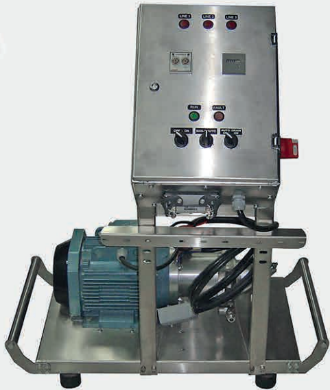
DFP6.3-8 8 LPM 100 BAR DANFOSS 230 V 54 Kg ALL SS FRAME Control Box, On-Off timer, Pressure Switch, Automatic Drain
